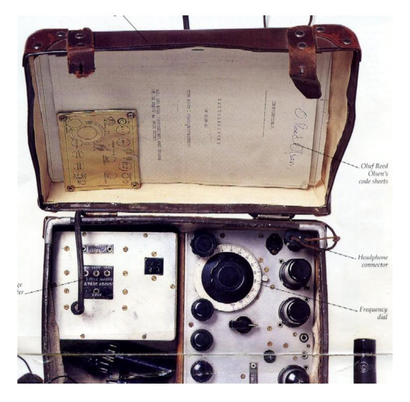
This particular Paraset also has a 6 VDC power supply included with it which connected to a car battery via large alligator type clips. The switch is the 80/40 meter bandswitch. There is also a nice all-brass key connected to the rig out of the photo to the left . The plain black knob just below and a little to the right of the band-switch is the emergency key. The pointer-type knob near the center is the transmit-receive switch.
