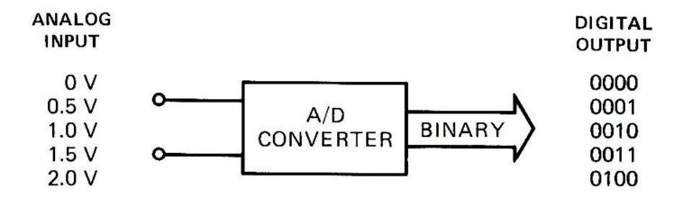
The A/D or ADC samples an analog voltage at various points.
