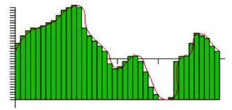
Therefore, in order to digitize the analog data accurately, we need to sample the analog signal as fast as possible with an A/D that has large number of bits.
