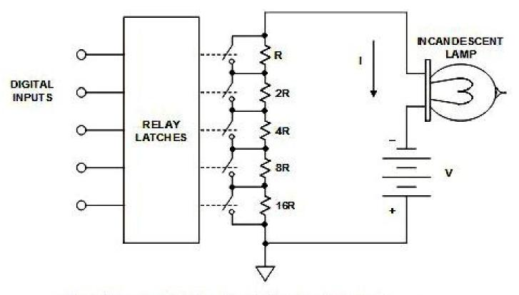
Adapted from: Paul M. Rainey, "Facsimile Telegraph System," U.S. Patent 1,608,527, Filed July 20, 1921, Issued November 30, 1926 A resistive network can be used as a *binary ladder* in a DAC, whose output voltage  $V_A$  is a weighted sum of the digital inputs.
