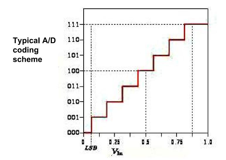
The analog signal is continuous in time. But, it's necessary to convert this to a flow of digital values.
